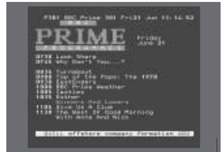
A typical Teletext page. The current page number, channel name, date and time appear at the top of the screen, as well as a three-digit number showing the progress of the page search function.
