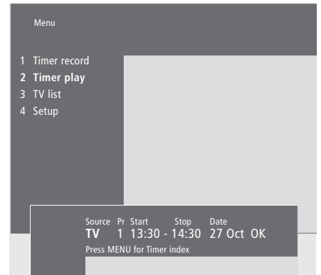
The Timer Play menu. To see previously entered timer settings, press MENU...
