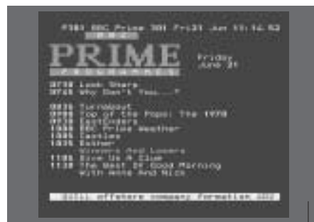
A typical Teletext page. The current page number, channel name, date and time appear at the top of the screen, as well as a three-digit number showing the progress of the page search function.
