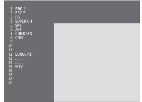
The TV channel list. Dotted lines show that a channel has been stored, but not named. An empty slot in the list shows that no channel has been stored there.
