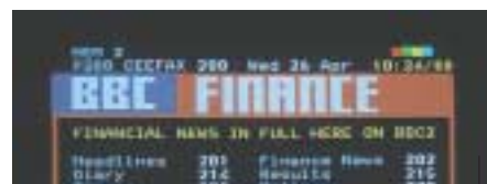
A Teletext page with the colour bar at the top right indicating that it is a Fasttext page.
