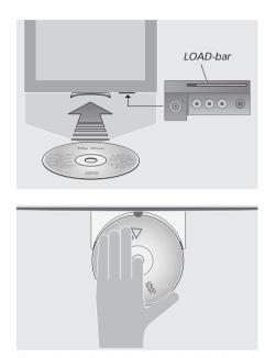
Place a disc in the loader so that the side edges of the disc rest on top of the loader's side pads while the front edge rests under the loader's front pad.
