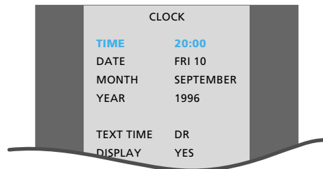
Menu for setting the clock – the item TEXT TIME indicates synchronisation with Teletext. The item DISPLAY indicates whether or not the clock will be displayed on the BeoCenter AV5 display
