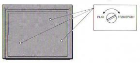
Before using the record player you must loosen the three transport screws underneath it. Place the record player on a table, with its front protruding over the edge of the table. Hold the record player firmly and turn it carefully until you have located and loosened each screw. The screws cannot be removed from the holes but should be turned several times using a screw-driver or a coin.
