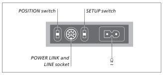
The socket panel is located on the bottom part of the loudspeaker.
