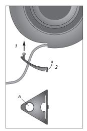
Cover for socket panel: Run the two cables through the hole (A), before you connect them to the loudspeaker.
