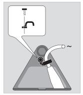
Cable Clamp: For safety reasons, the mains lead must be secured to the loudspeaker. Use the enclosed small cable clamp and screw.
