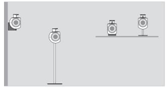
The loudspeaker must be placed on either the black rubber base, a floor stand, a table stand, or a wall bracket.
