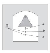
The mounting holes (b and c) are blocked by two small screws, and before you can use either of these holes, the screw must be removed.
