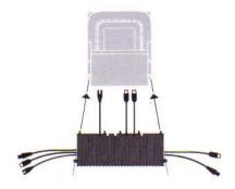
Note: Additional cables, for examble from auxiliary equipment, may also be run behind the cable cover, together with the existing cables. If you want to do so, you must connect the equipment to the Beosystem 2500 before you fasten the cable cover to the centre unit.
