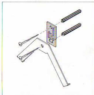
*The enclosed accessories must be used only when mounting the loudspeakers on solid walls.*
