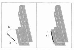
Fasten the cable cover to the grill on the Beocenter rear panel:
