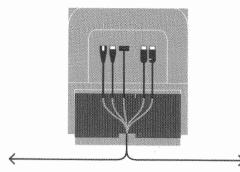
Arrange the connector cables in the cable cover as shown above.
