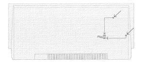
The Beocenter is provided with two screws on the base which protect the compact disc unit suspension during transport. These screws must be loosened before you can operate it. To gain access to the screws carefully turn the Beocenter upside down. Remove the two screws with a screwdriver and place them in the two holes marked PLAY for safe keeping.
