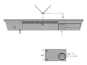
Before connecting the Beocenter to the mains, check that the mains voltage switch on the rear panel is set to the position corresponding to the voltage supply in your country: **220** V, **130** V, **240** V, or **110** V.
