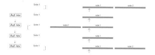
During this step procedure the current side is played unaffected, as indicated by the cue **Side 1** which remains lit all the time. If you are on side 2 of the tape, the same cycle can be passed through, but in reverse order and with **Side 2** lit instead.
