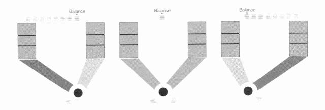
If you are adjusting balance, pressing shifts the sound towards the left-hand speaker, pressing shifts the sound towards the right-hand speaker. This function enables you to direct the sound emerging from the loud-speakers towards your favourite listening position.
