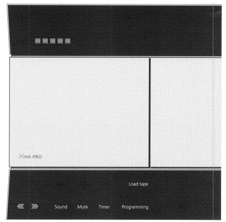
The first group or level of controls are accessible at all times. They are identified by light grey print and are for selecting source, adjusting sound levels and programming.
