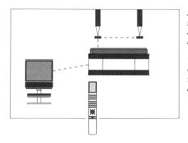
All that is required for the integrated audio/video system to work is that your Bang & Olufsen audio and video systems are interconnected by a special link cable.
