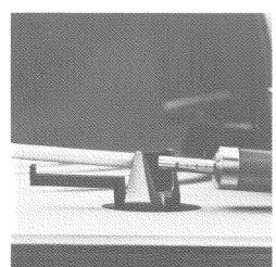
pickup arm should now »float« with respect to the black suspension fork.
