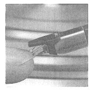
**Stylus guard** Flip up the stylus guard.
