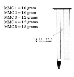
If you want to check the stylus pressure using a stylus gauge, place the gauge underneath the stylus, press LIFT> and keep the button depressed for more than two seconds. The tonearm will then lower onto the gauge, and you can read off the pressure on the gauge.
