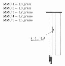
If you want to check the stylus pressure using a stylus gauge, place the gauge underneath the stylus, press  $\rightarrow$  and keep the button depressed for more than two seconds. The tonearm will then lower onto the gauge, and you can read off the pressure on the gauge.
