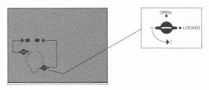
If you ever have to transport the compact disc player, we strongly recommend that you reinsert both the cardboard protecting the disc tray and the two transport screws.
