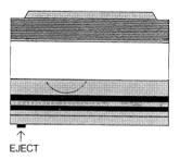
If the compact disc player is not connected to the mains, the dust cover will not open, when you press the EJECT button. However, the lock mechanism will be released so that you can open the cover manually.
