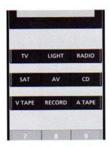
The Source buttons (TV, SAT, V TAPE, RADIO, CD, A TAPE, LIGHT and AV)... are used for switching on your Bang & Olufsen audio and video products as well as audio/video integrated system and the Bang & Olufsen light control.\*
