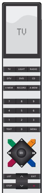
Source buttons and buttons for recording.
