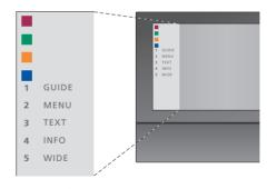
Example of a Set-top Box Controller menu – The Beo4 buttons are shown to the left on the menu and the set-top box buttons are shown to the right.
