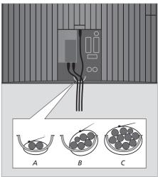
IMPORTANT! All the cables must be fastened to the television using the enclosed cable tier as shown.
