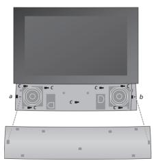
Attaching the speaker cover: Hold up the speaker cover slightly to the right of the 'brackets' a and b. Now slide the cover to the left to let the 'attach-points' engage with the corresponding 'brackets' (a, b and c) on the television.
