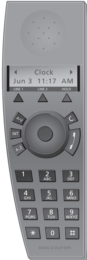
The display is illuminated when the handset is in use.
