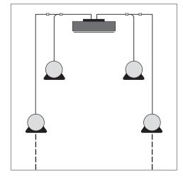
The special adaptor, part no. 6270706, can be used to connect additional pairs of BeoLab 8000 speakers to your Bang & Olufsen system. The adaptor is available as an optional accessory from your Bang & Olufsen dealer.
